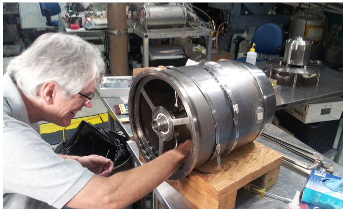
Photo 2) Bill successfully installs the sensors in the actual titanium UPA drum at the NASA Marshall Space Flight Center – within the allotted time and budget.
